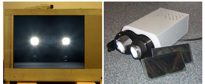
Figure 2: The HDR Display (left) and the HDR Viewer (right). Both devices are capable of contrast ratios in the region of four orders of magnitude.
