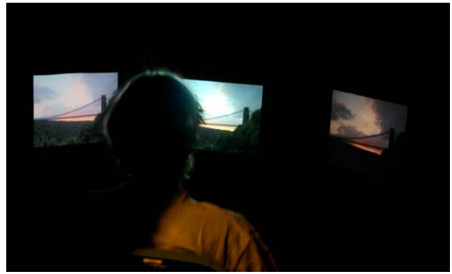
Figure 2: Experimental setup. In the center is the linearly mapped reference image on the HDR display. Left and right are two tone mapped images.
